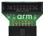
Figure 2-9: JTAG 14-way Texas Instruments adapter
